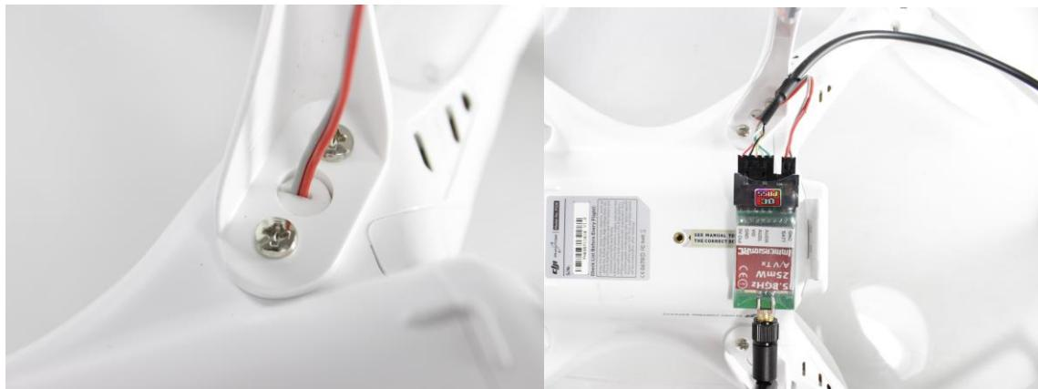
Every Phantom has such a power cable installed out of the box, which can be used for e.g. video transmitters. This cable is assembled without any connection plug. You can pull it out a few inches if you remove the white rubber plug, please push the plug back in gently afterwards. To connect to the transmitter, you can either crimp suitable connectors on the cable if you have them at hand, or use the power cable which comes with the transmitter.
