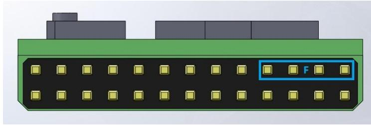
This port is used for the optional telemetry data radio.
