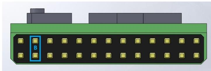
PIN#2 is connected with PIN#1 internal. PIN#15 is the power supply pin for Camera and VideoTX.
