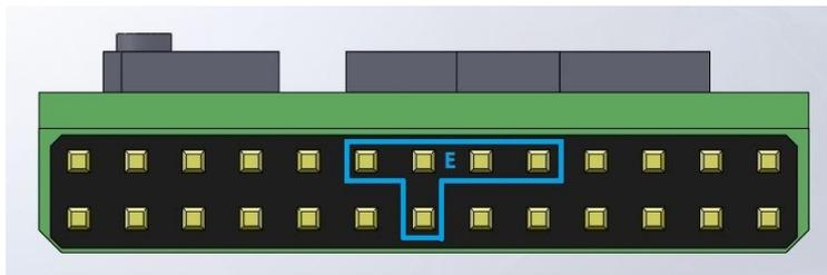
This port is for current sensor, battery voltage sensor and RSSI input.
