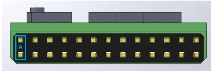
This port supplies power to the TFPro. The TFPro has its own switching power unit so it can be powered from 7-20V. But if you want to share this power with the camera and the video transmitter, we recommend you to power the AP with a 3S lipo since most of the camera and video TX need 12V.
