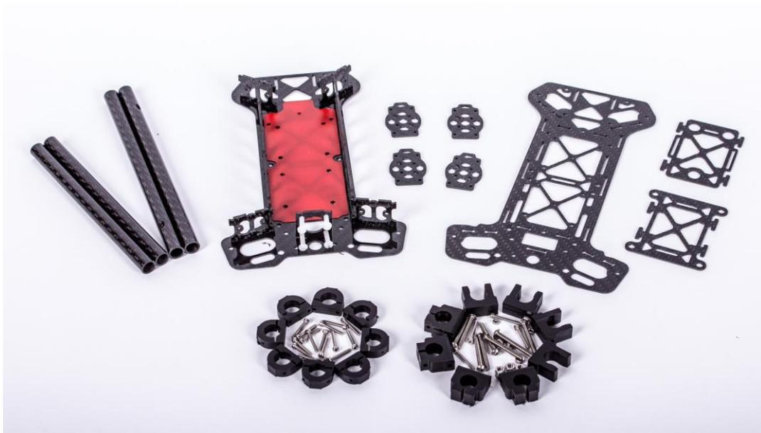
We recommend that you test-fit all components first, the long booms should be mounted to the rear end and the short booms to the front end. Doing so, you can measure the approximately required cable length und cut them.
